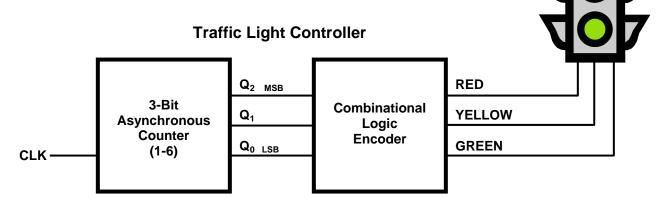
Your task is to design the two sub-systems that make up the complete traffic light controller that meet the following design specifications.
